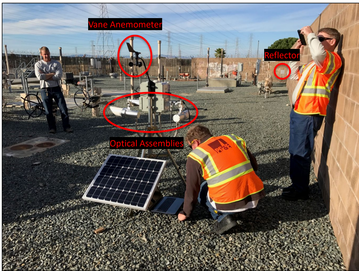
Sensit FPL unit set up at a Transmission Station in Pittsburg
