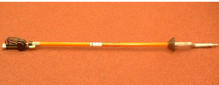
The long-handled lance features an articulating head to facilitate safe excavations around the circumference of buried pipes.
