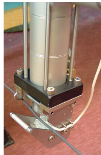
ESI pneumatic handle and attachment for tracer wire connection
