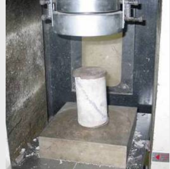
Slant shear & punch out tests
