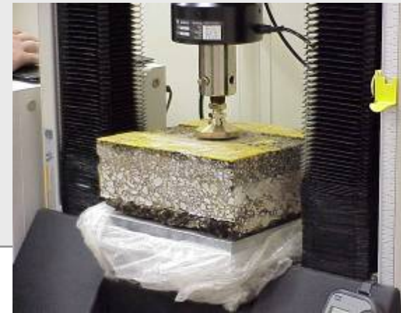
Slant shear & punch out tests
