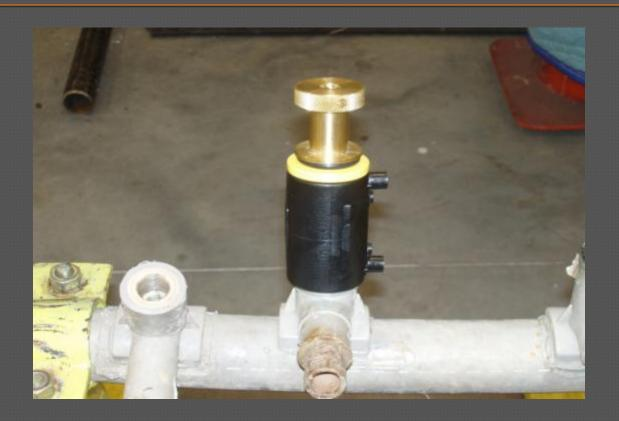
After removing the electrofusion control box cables, allow the electrofusion coupling and insert assembly to cool for a minimum of **10 minutes** before further assembly work.
