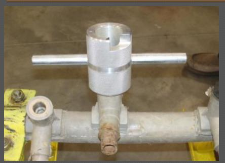
Scrape outside diameter of tee stack with side "A" facing down on the Scraper/Peeler tool (beveled side down).
