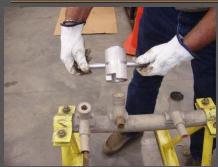
The outside diameter of the Aldyl-A tapping tee shall be scraped until side "B" of scraper is touching the intersection of the tee outlet.
