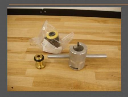
Standard Kerotest Aldyl-A Tapping Tee Repair Kit Peeler for scraping Aldyl-A Tee Insert Holding Tool (p/n 72770524)
