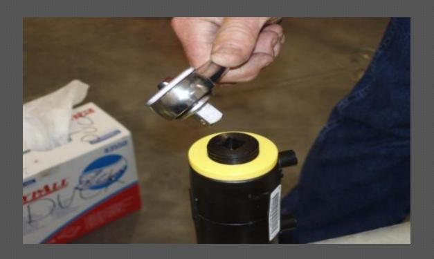
Use a standard  $\frac{1}{2}$ " square drive to turn the plug into the Insert. The top of the Plug should be flush with the top of the Insert.
