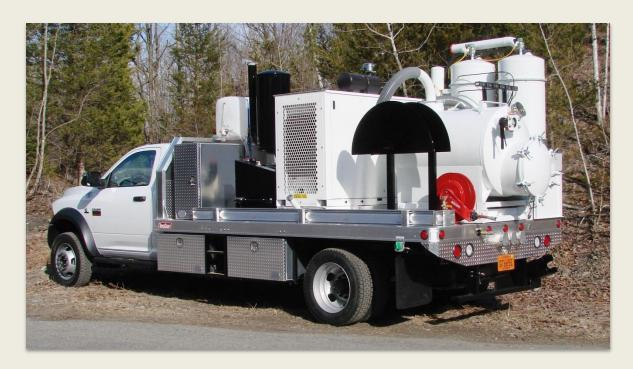
Gas evacuator systems can be used with any vacuum excavation that is equipped with a 4" diameter vacuum digging hose and has the ability to produce a flow rate from 780 to 1,100 SCFM.
