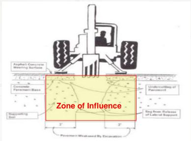
Zone of influence is the area around the excavation that is susceptible to slippage or collapse resulting from external surface load, from vehicles, plant, or excavated material at or near the excavation.
