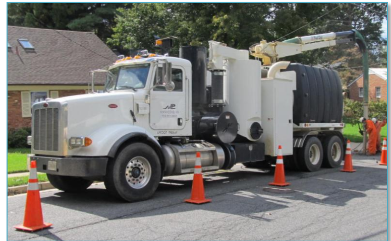
Hydro-Vac with 1800 gallon water tank and 10.6 cubic yard storage capacity
