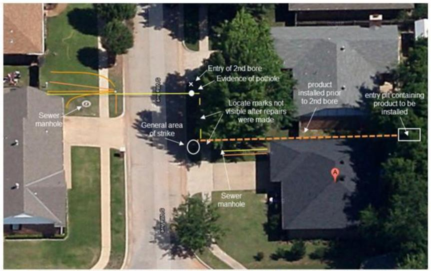
Aerial view of area prior to explosion obtained from Google Earth and revised with site information. marked phone/cable line marked natural gas line phone line installed by contractor prior to 2<sup>nd</sup> bore Oklahoma City – January 2013 Sub-contractor installing telecom lines parallel to gas line Injuries and house destroyed
