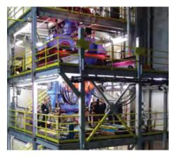
multiple points. The splitter system uses a GTI proprietary ultra-dense pneumatic conveying system that has been developed to minimize gas requirements for transport.
