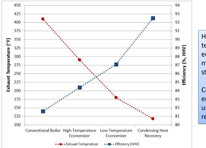
High and low temperature economizers may be made of carbon or stainless steel
