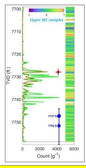
Proppant height of only 30' in Upper Wolfcamp - 5% of Microseismic height
