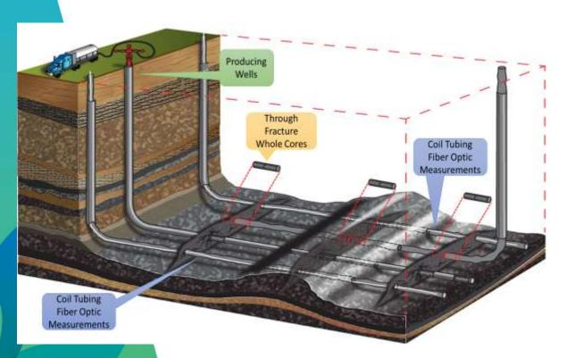
Ground Truth: Through-Fracture Cores
