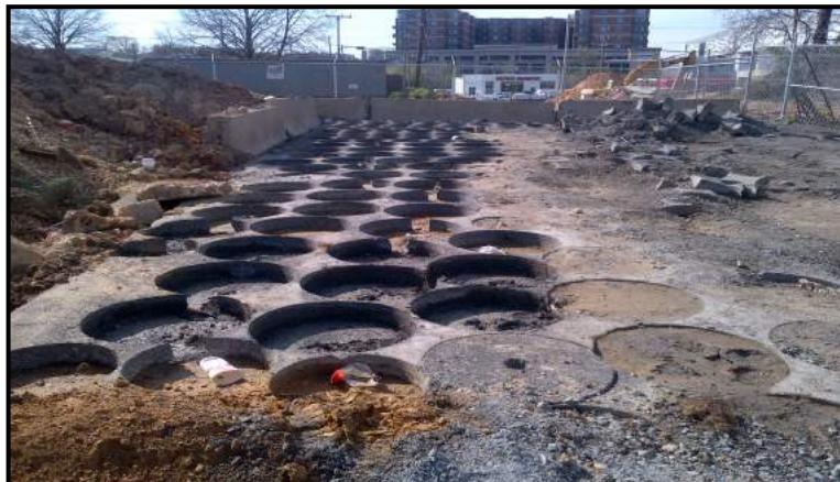
A Core Farm where cores can be harvested year around as needed to replace defective cores from the field.
